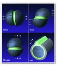
Adhesive tapes have been developed to withstand a variety of forces on the bond. As a rule, tapes perform better when the primary stress is tensile or shear. Most industrial applications involve a combination of stresses.
